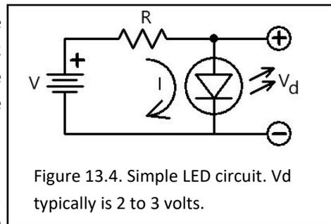
Figure 13.4. Simple LED circuit.  $V_d$  typically is 2 to 3 volts.
