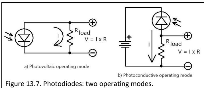
Figure 13.7. Photodiodes: two operating modes.
