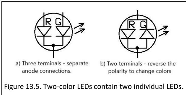
Figure 13.5. Two-color LEDs contain two individual LEDs.
