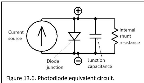
Figure 13.6. Photodiode equivalent circuit.
