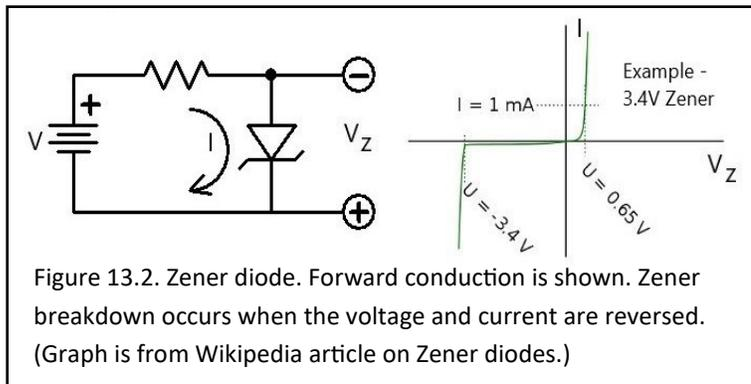
Figure 13.2. Zener diode. Forward conduction is shown. Zener breakdown occurs when the voltage and current are reversed. (Graph is from Wikipedia article on Zener diodes.)
