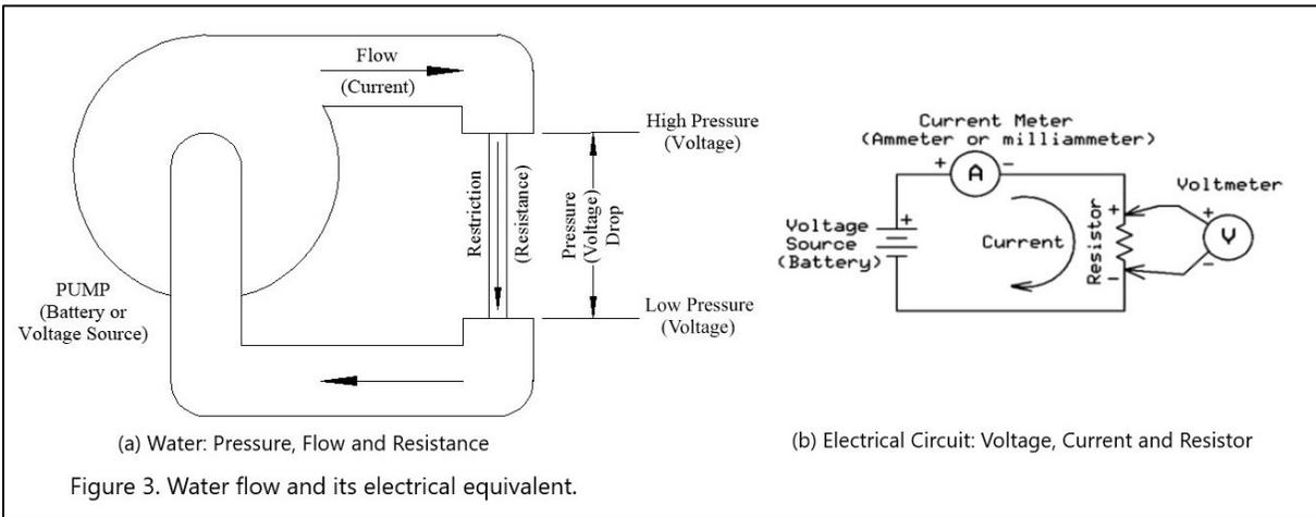
Figure 3.1(a), repeated from the previous chapter, shows this using water flow. The pump provides pressure, forcing the water to flow through a restriction. The restriction resists the flow of water: the smaller the restriction, the lower the flow. Flow through the restriction causes a pressure drop, or difference.
