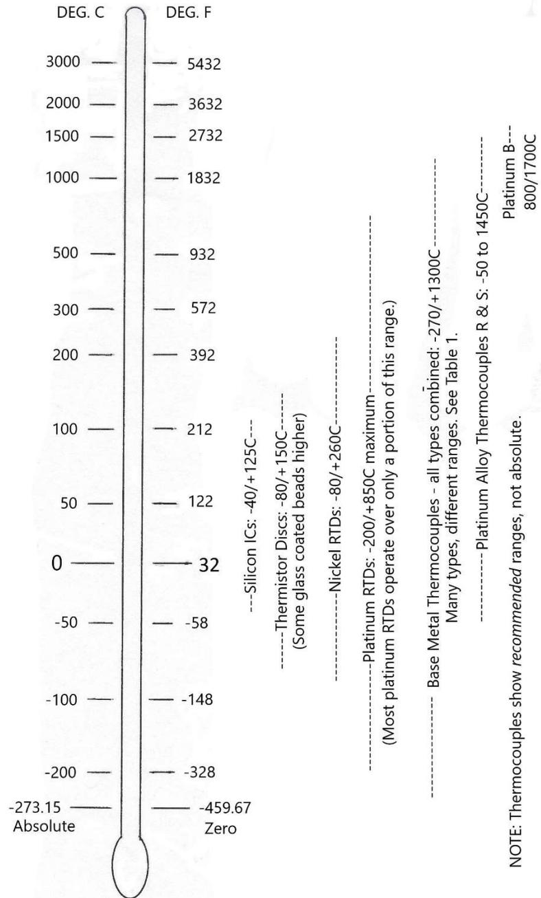
Figure 1: Typical Temperature Sensor Ranges.
